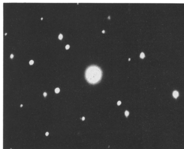
Figure 5 HTREM micrograph of the Ag/Si (111) interface. Compared with Fig. 4, silver is slightly rotated around the [110] axis.
